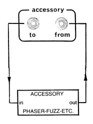
The accessory "to" output provides easy patching of external accessories such as echo, phasers, and etc.
