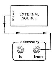
Occasionally, you may find it necessary to use your Alpha 112 as a power amp. Using the patch guide only that program from your external unit will be amplified to the speaker.
