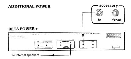
The accessory "to" output is utilized for driving additional power amplifiers from your Alpha System. Calibrated for the Beta Power + or Alpha Slave, but still compatible with other slave amplifiers.
