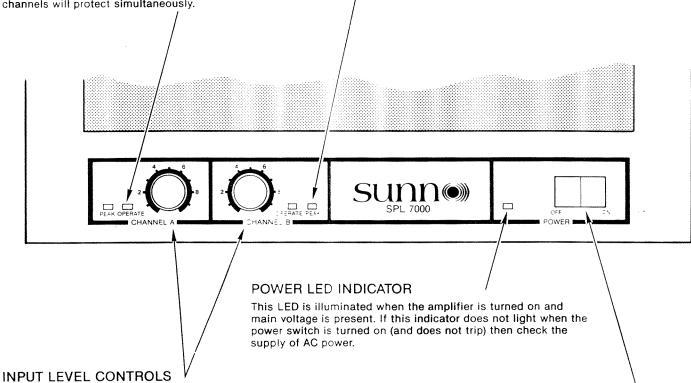
Two (2) 41-position attenuators that control the amplifier input sensitivity. The control settings can vary between zero attenuation or loss (sensitivity is +4dB/1.23VRMS) and infinite loss (at least - 85dB from maximum sensitivity). The controls are detented (click-stepped), making them accurately resettable. A separate control is provided for each channel. When operating in the Bridged Mode only the Channel A control is active (the Channel B control has no function). Refer to the
