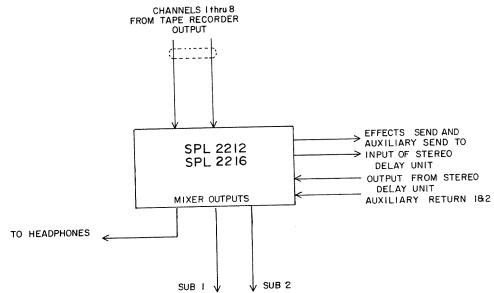
TO LEFT AND RIGHT POWER AMPLIFIERS OF STUDIO MONITORS, AND LEFT AND RIGHT CHANNELS OF STEREO RECORDER DIRECTLY OR VIA A NOISE REDUCTION UNIT OR COMPRESSOR.
