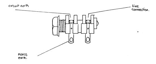
The wiring above enables the mains earth to be disconnected when an audio lead is inserted into the jack
