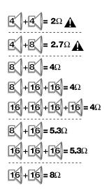
Generally, you will want to connect your amplifier to speakers with a total impedance load equal to the minimum impedance rating of your amplifier. A Operating below the minimum impedance rating can easily overheat the amplifier and cause damage. Operating above the minimum impedance rating will reduce the amplifier's maximum power output.
