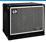
1x15 enclosure, 200 watts handling, custom SWR® speakers, piezo tweeter with attenuator, Speakon® and 1/4" speaker jacks, side handles, chrome-powder coated shock-mounted grill, front slot port. 60 lbs. (27.22 kg) Impedance: 8 ohms.
