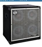
4x10 enclosure, 400 watts handling, custom SWR® speakers, piezo tweeter with attenuator, Speakon® and 1/4" speaker jacks, removable casters, side handles, chrome-powder coated shock-mounted grill, front slot port. 97 lbs. (44 kg) Impedance: 4 or 8 ohms.
