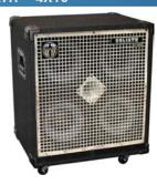
4x10 enclosure, 800 watts handling, custom SWR® speakers, horn tweeter with attenuator, Speakon® and 1/4" speaker jacks, removable casters, side handles, vibration-free shock-mounted chrome grill, front slot port. 89 lbs. (40.37 kg) Impedance: 4 or 8 ohms.
