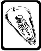
Tube life varies depending upon playing style and application. Power tubes have a much shorter life than pre-amp tubes which can last for years. For continued optimum performance from your amplifier, the tubes should **ONLY** be replaced with
