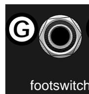
**G. FOOTSWITCH** - Plug-in connection for the footswitch (P/N 053895) used to remotely turn on and off the graphic equalizer, compressors and change the channel selection. Using the footswitch will override the front panel graphic equalizer, compressor and the channel selection buttons. *NOTE: Any good quality patch cord will work with the remote footswitch, however an unshielded speaker type cord is preferable to a coax guitar cord.*
