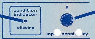
Input Sensitivity control allows the user a wide range of input amplitude. When used with a Beta Lead or Bass, the sensitivity control would normally be set at maximum. This calibrates the Power+ to the Lead and Bass for the same output level.
