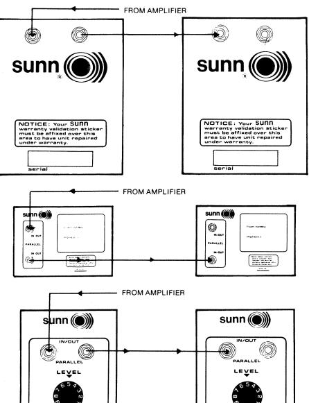
For Sunn enclosures that are provided with parallel input jacks, use either jack for the input, use the other jack to connect another enclosure in parallel. See the chart in the Series and Parallel section of this manual to determine the resulting impedance.
