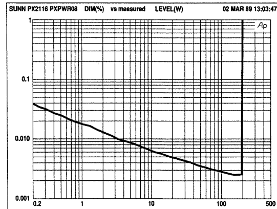
Figure 3-22. DIM100 Distortion vs Output Power into 8Ω AMP IN to SPEAKER OUTPUT.
