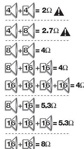
This illustration shows the total impedance loads of various combinations of speakers connected in parallel. Ideally, you will want to connect your amplifier to speakers with a total impedance load equal to the minimum impedance rating of your amplifier. Operating below the minimum impedance rating can easily overheat the amplifier and cause damage. Conversely, operating above the minimum impedance rating will reduce the amplifier's maximum power output capability.
