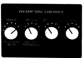
TREBLE LEVEL control and PULL FOR BRITE - The TREBLE level control obviously increases the treble response of the STP-G II preamp stage. However, it also functions as a pull-switch to activate the Brite circuitry for extra edge.
