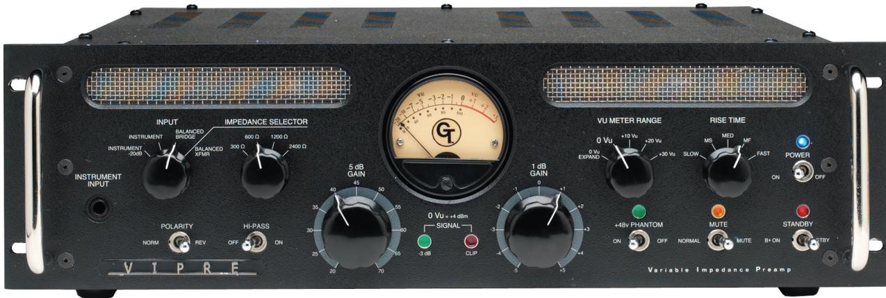
**VARIABLE IMPEDANCE INPUT** Custom-wound transformers load mics at 300, 600, 1200 or 2400 ohms, multiplying the performance potential of every microphone. Additional transformerless balanced bridged, line and instrument inputs.
