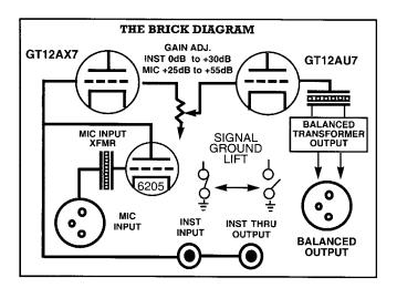
NOTE: The balance output signal from the Brick uses Pin 2 as "hot", consistent with the AES standard. You may "unbalance" this signal and run it single ended but hum and noise induction may result depending on the environment conditions.
