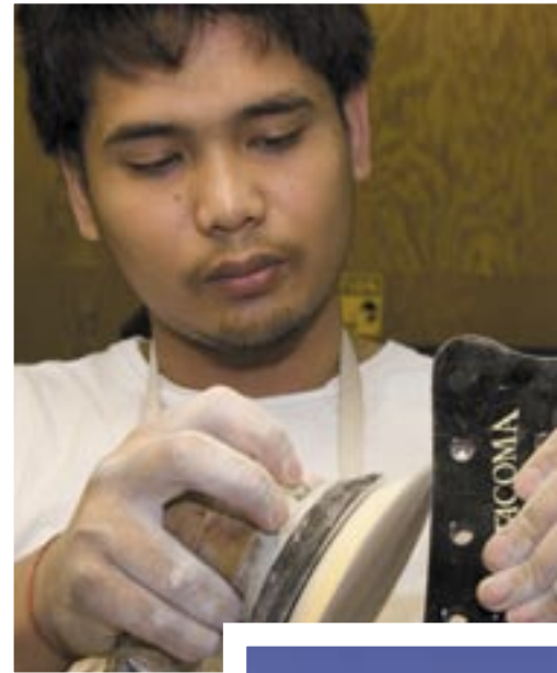
NECKS ARE SHAPED AND SANDED FOR THEIR FAST MODERN FEEL (ABOVE).
