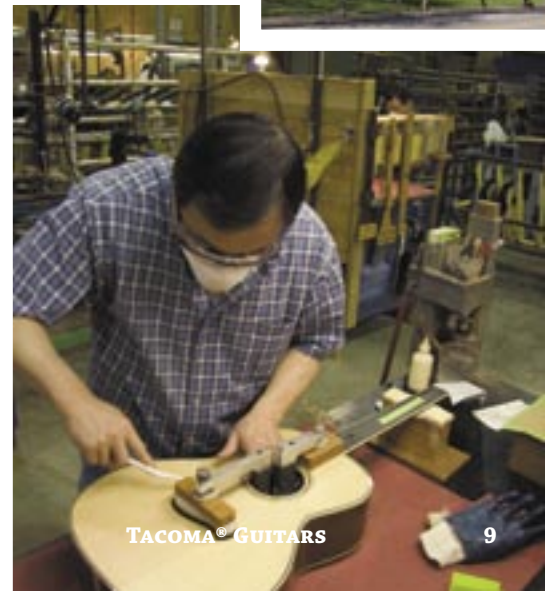
OUR PROPRIETARY BRIDGE IS GLUED TO AN ALL-SOLID SPRUCE TOP (BELOW).
