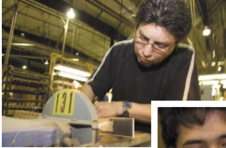
NECKS ARE SHAPED AND SANDED FOR THEIR FAST MODERN FEEL (ABOVE).
