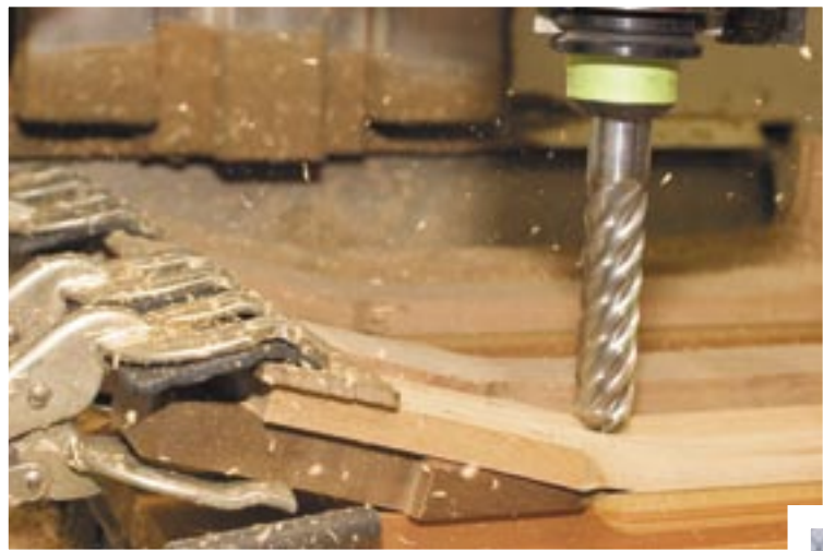
SELECT NORTHWEST HARDWOODS BEING MILLED (BELOW) TO BECOME NECKS, AND DRILLED (ABOVE) FOR TRUSS ROD INSTALLATION.
